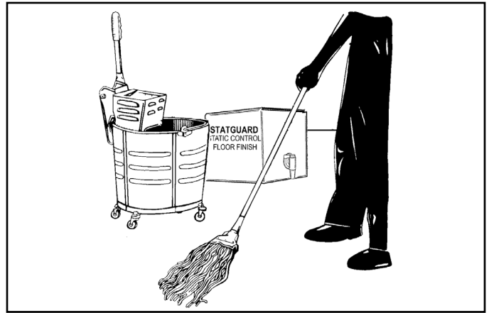
Figure 4. Applying floor finish
