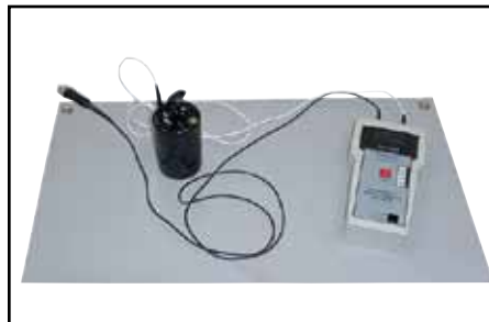
Figure 2. Testing RTG with Surface Resistance Test Kit.
